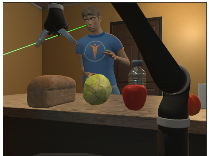
Fig. 1. The robot’s perspective when prompting the user for a description of the bread. The gaze line (not visible to participants) is overlaid on the image as transformed from the virtual reality headset’s tracking to demonstrate the gaze-to-object proximity visible from the robot’s sensors.
