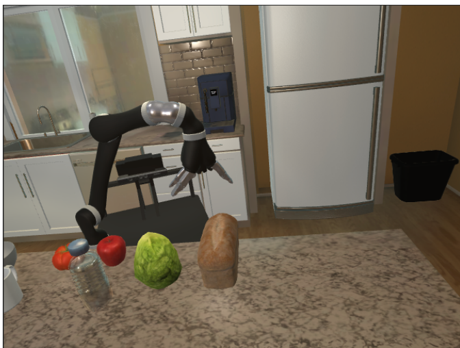
Fig. 2. The user’s perspective of the robot moving its arm over the bread to ask the user for a description. The robot’s audio informs the user of the robot’s desire to know about the object and the movement of the arm indicates which object is of interest.
