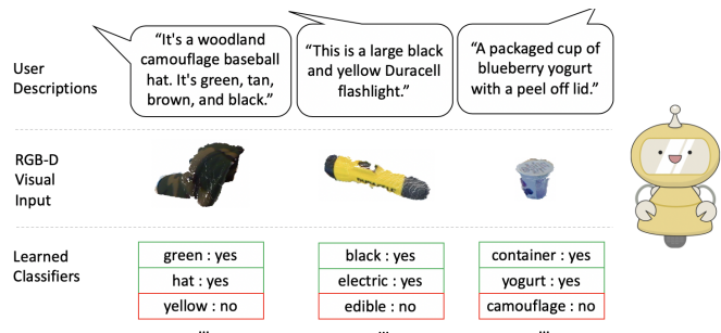
Fig. 1: Examples of object descriptions from Amazon Mechanical Turk workers above RGB point clouds. The robot then learns classifiers for each concept and whether they relate to the given visual input. Note the correct application of concepts not explicitly present in class labels, e.g., electric , which is learned solely from user descriptions.
